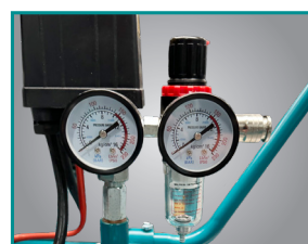
Filter pressure regulator for infinitely variable adjustment of the working pressure, with simultaneous dirt, oil and condensate separation
