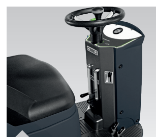
Mechanical operation of the brushes and suction bar via levers
