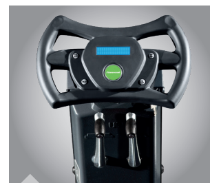
Electronic control panel with diagnostics and 2 levers for the side brushes
