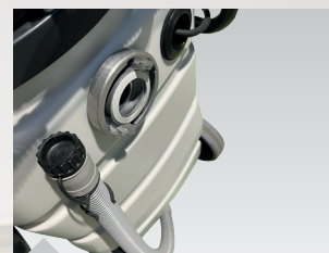
Connection of the fire hoses via C-coupling (Storz coupling, non-return valve is in the tank)
