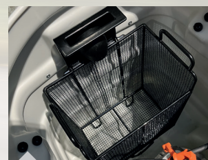
Dirt trap separates solids from liquids, protects the pump and facilitates disposal. It effectively protects against blockages caused by stones, leaves or wood that have been sucked in
