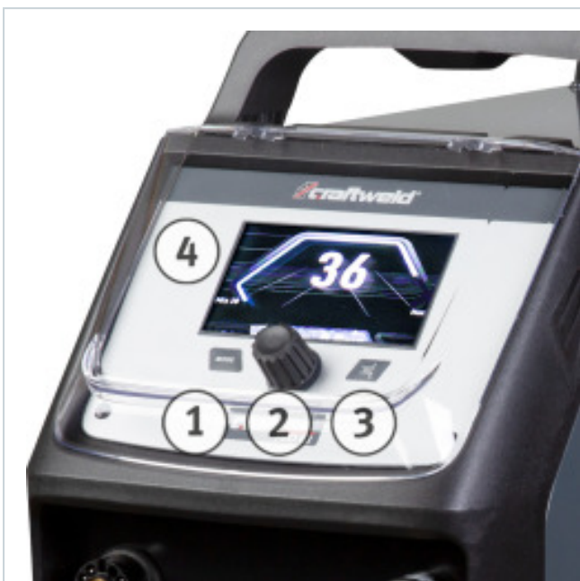
Function button for setting 2-stroke, 4-stroke, perforated sheet metal Control for setting the current intensity Compressed air test Digital display
