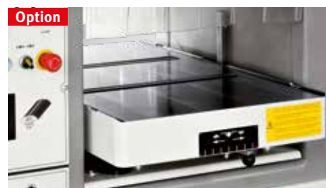
Option two rollers in the thickness table
