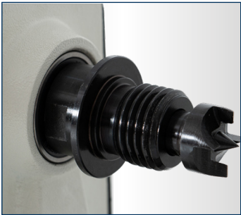
• Spindle with ASR safety catch. Prevents the clamping device from "running off" in conjunction with the retaining ring available as an accessory
