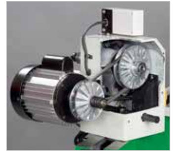
Vario speed regulation from 500-2000 min -1 via V-belt and adjustable conical pulleys
