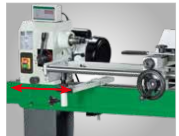
The headstock can also be moved sideways and locked at any point on the lathe bed
