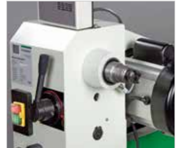
The desired speed can be set quickly and easily using a lever on the operator side
