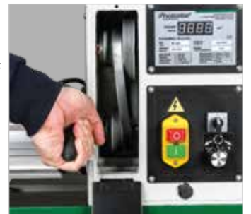
Tool-free changing of the transmission ratio by simply remounting the V-belt
