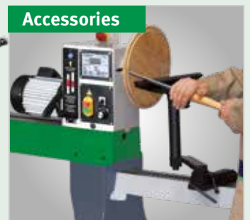
The headstock can be swivelled to turn workpieces in cross-grain operation that are larger than the bench's turning diameter. The bed extension in combination with the reversible tool rest enables maximum flexibility.
