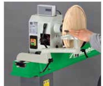
The headstock can be swivelled to turn workpieces in cross-grain operation that are larger than the bench's turning diameter. The bed extension in combination with the reversible tool rest enables maximum flexibility.
