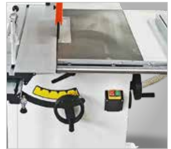
Saw blade height and tilt conveniently adjustable via handwheels
