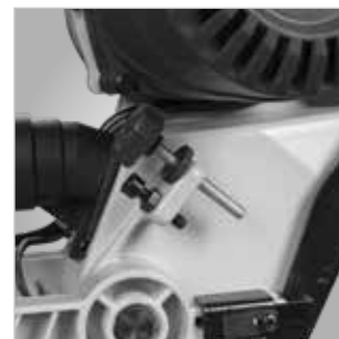
Double adjustable cutting depth limiter
