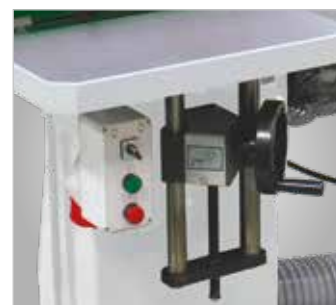
Height-adjustable sanding table for the utilisation of the entire sanding belt width
