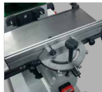
Angle stop adjustable by 60° on both sides
