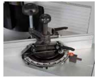
Infinitely adjustable angle stop
