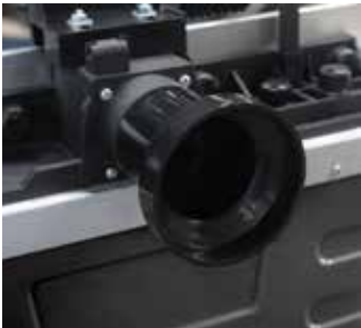
100 mm connection piece for external extraction
