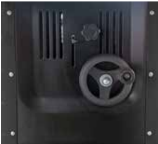
Spindle height adjustable from 0 to 40 mm
