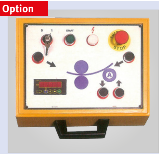
Control panel with digital display for side roller, motorised adjustment of side roller and button for material feed instead of foot pedal (optional)
