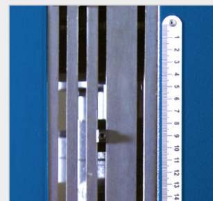
Upper and lower end position of the piston stroke as well as switchover point from rapid traverse to press traverse infinitely adjustable via cam ledge
