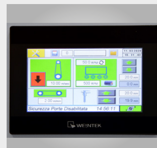
Operation of machine functions via 8" touchscreen
