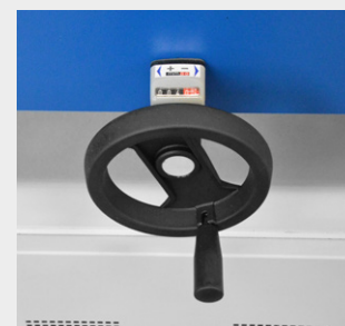
Manual height adjustment of the worktable with numerical display
