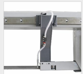
Cooling system directly on the saw blade guides Your benefits: High service life of the saw band with a clean cut
