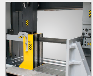
Front band guide moves parallel to the movable clamp jaw – resulting in more precise saw band guidance
