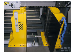
Clamping of the material before and after the cut by means of a two-part clamping block
