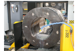
Clamping of the material before and after the cut by means of a two-part clamping block
