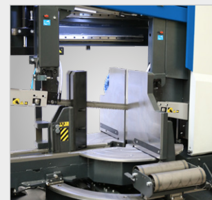
Turntable with lateral material support rollers
