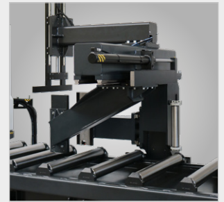
2000 mm roller conveyor and material transport
