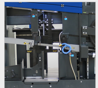
Saw band inclination of 7° and hydraulic saw band tensioning increase the service life of the saw band
