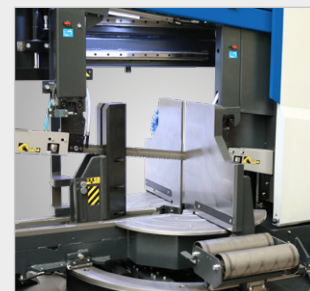
Turntable with lateral material support rollers
