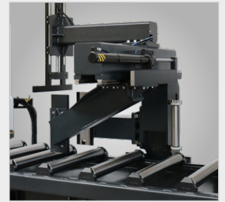
2000 mm roller conveyor and material transporter
