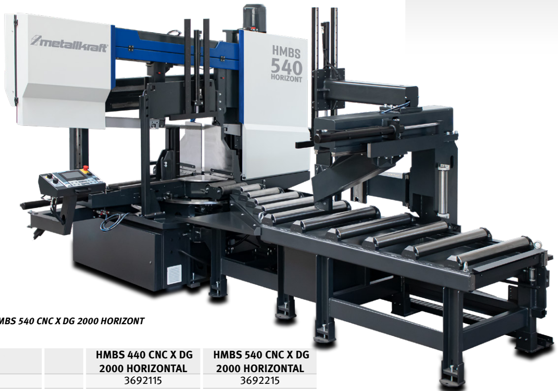
Turntable with lateral material support rollers
