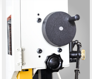
Height adjustment of the saw blade guide by handwheel
