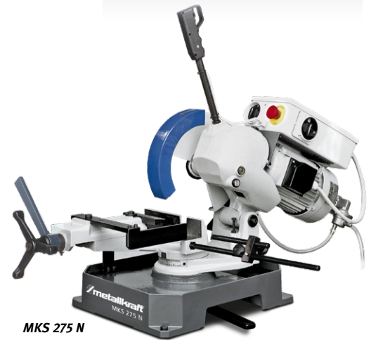
Quick-action clamping vice can be swivelled 45° to the left and 45° to the right
