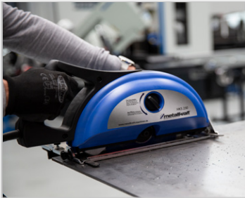
Double-guided rip fence for precise cutting
