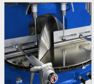
Stepless adjustment of the mitre angle
