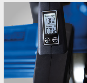
Digital Display. For displaying the saw blade speed, among other things
