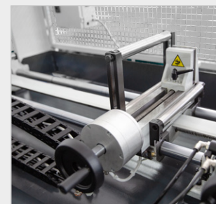
Transversely adjustable pneumatic quick-action vice
