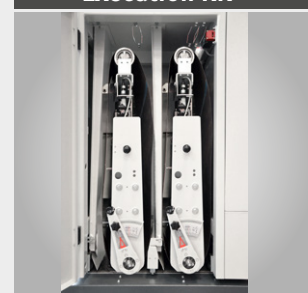
Two grinding belt units For deburring and surface finishing
