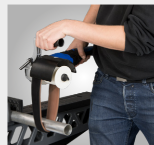
Satin finishing of round steel with Velcro fleece, even with already installed stainless steel railings, for example
