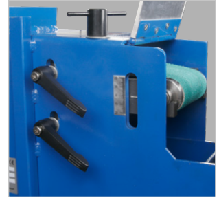
Simple, tool-free height adjustment of the grinding belt
