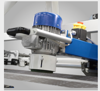
Disc grinding unit for selective machining, e.g. polishing weld seams
