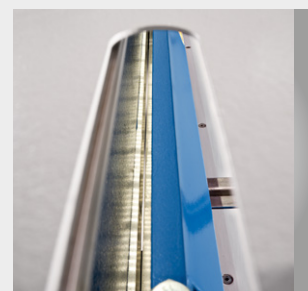
LED cut line lighting and viewing slits
