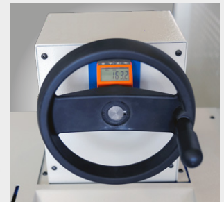
MTBS 2103 F / MTBS 3102 F Operation of the backstop from the front of the machine via handwheel and counter
