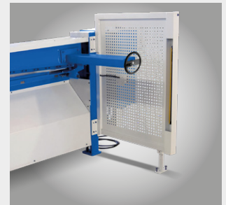
Rear area secured by light barrier
