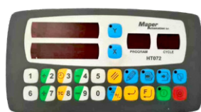
Positioning control for backstop Maper HT071
