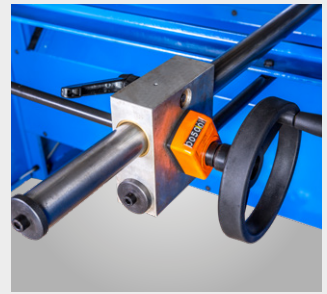
Manual back gauge 630 mm with millimetre-precise adjustment option
