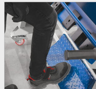
Quick foot clamping (short stroke approx. 20 mm)
