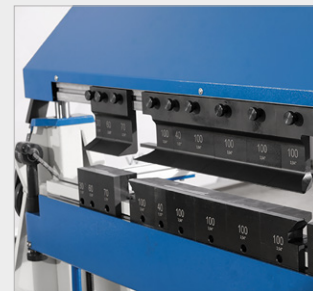
All three tools segmented and with quick-change system
