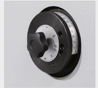
Serial control MA - manual adjustment of the bending angle using the scale ring on the left-hand side
