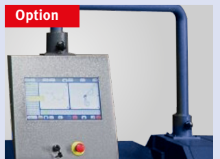
Optional CNC control with 3D graphics, the profiles are drawn by the operator on a large 19" touchscreen, all axis positions and the bending sequence are calculated by the control, motorised rear stop with stop fingers, travel range 10-1000 mm
