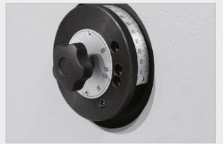
Standard MA control system - manual adjustment of the bending angle using a scale ring on the left-hand side of the machine
