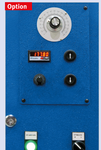
Optional PUD control with digital display, manual adjustment of the bending angle and adjustable motorised rear stop
