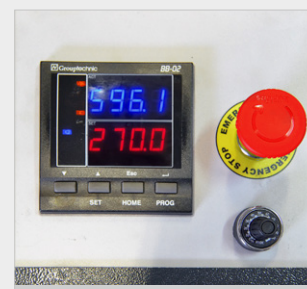
Simple operation, with digital display for current bending values and for setting the parameters
