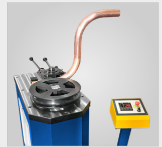
Bending angles up to 180° possible
