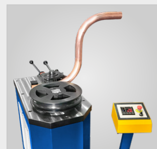
Bending angles up to 180° possible
