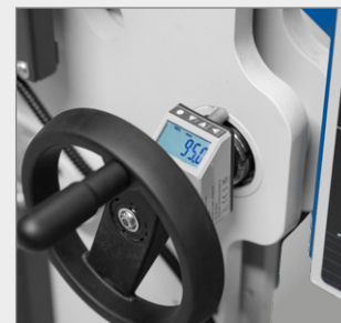
Adjustment of the rear stop via handwheel with counter
