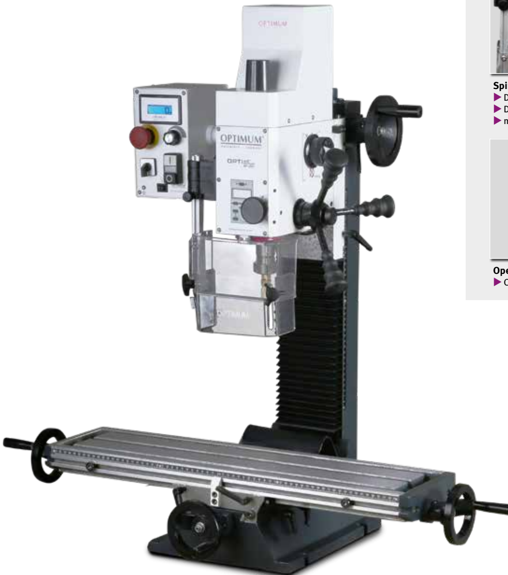
Fig.: OPTImill BF 20Vario with optional accessories milling
