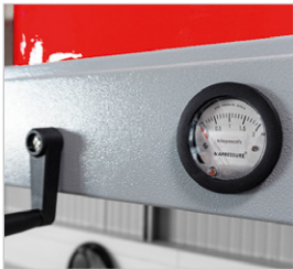
Filter monitoring via pressure gauge
