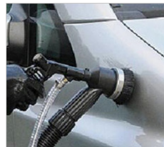
• Blasting agent is extracted and returned immediately after hitting the surface
